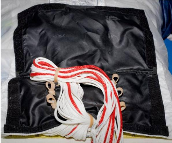
4) Begin stowing the remaining lines in the rubber bands on the tail pocket, starting with the bands at the top of the tail pocket (farthest away from the tail seam).
