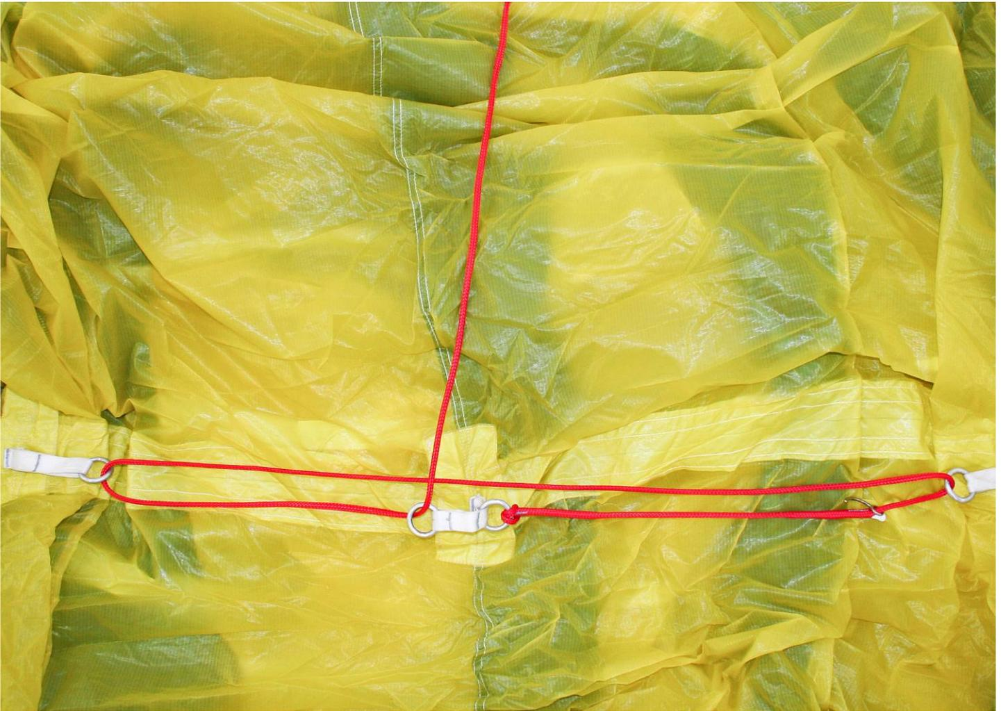
1. Take the looped end of the bridle closest to the white spur and run it through the lower ring on the center cell.
