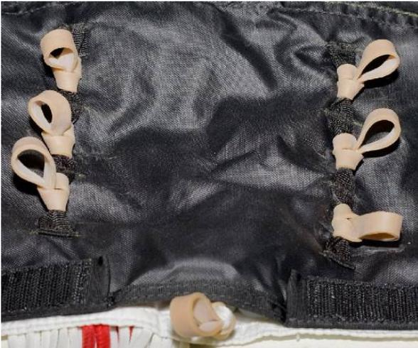
1) Attach a rubber stow band to the loop in the cavity formed between the tail of the canopy and the tail pocket. Add rubber stow bands to the loops inside the tail pocket.
