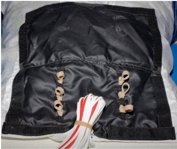
2) Make a single line stow in the band inside the cavity formed between the canopy and tail pocket as shown.
