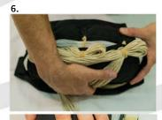
Rotate the bag forward on top of the lines and secure the side tuck tabs.
