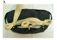
Center locking stows are to be made before moving along to the outer locking stows. All locking stows are to be free and clear of each other.
