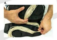
Open the line stow flap and route the excess suspension line over the top of the bag down to the bottom of the line stow flap. Begin creating figure 8 line placement starting at the bottom center of the line stow flap.
